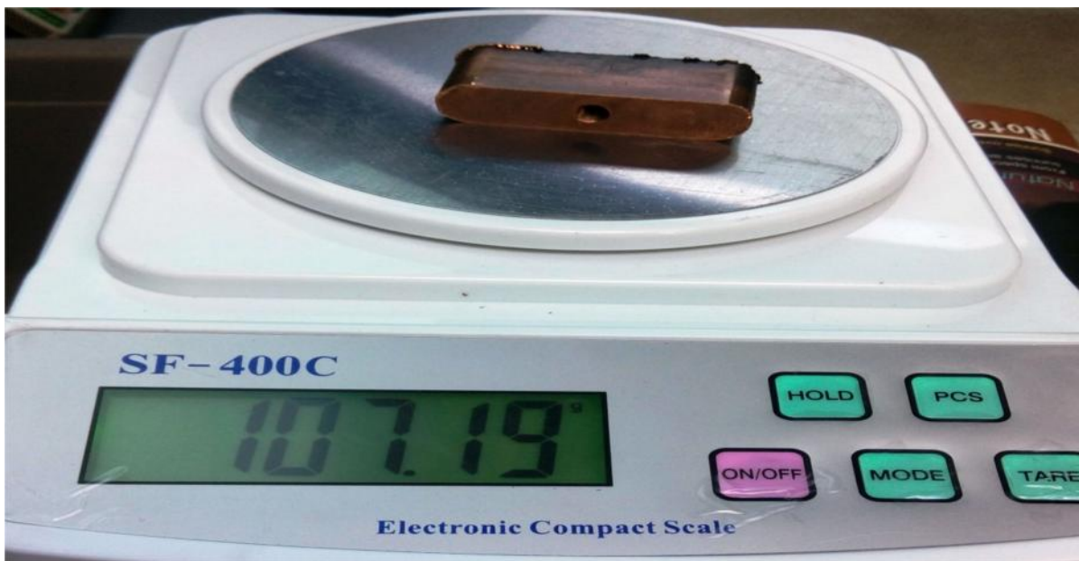
Figure 2: Weight measuring of Copper Electrode through Electronic Compact Scale
